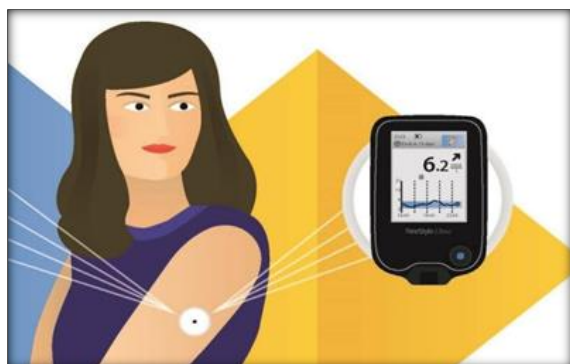
Figure 1: This cartoon shows the Sensor and the Reader and the information available on the screen on wiping the machine over the sensor
